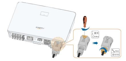
The fixed wiring is protected by a weatherproof shroud which is locked in place by a screw.
