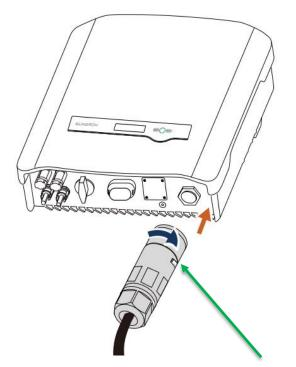
Push screwdriver into the slot to release the locknut.
