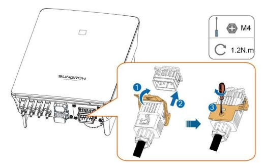
Unscrew the locking screw to release the plug locking device.
