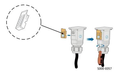
The AC plug is locked into place by the locking clip, and can only be removed with a screwdriver.
