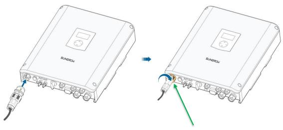
Push screwdriver into the slot to release the locknut.
