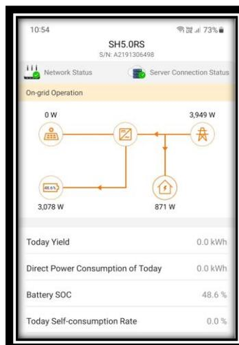
Picture 6 – Genset supplying loads and charging battery
