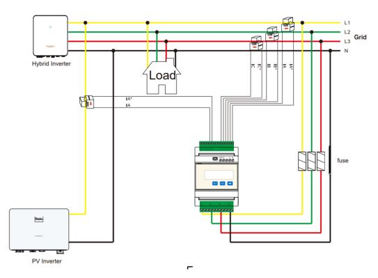
The primary CT(s) are connected at the top right of the meter, and clip over the incoming main(s).
