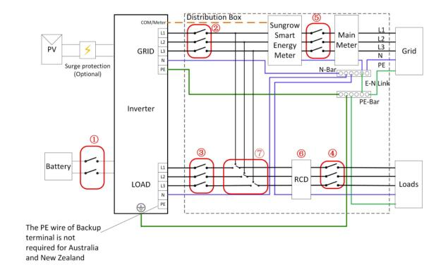
Earth the chassis as per above, and install the supplied 63 Amp changeover switch.
