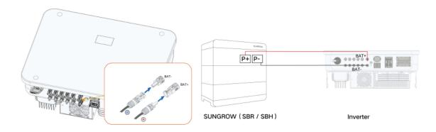
Insert the terminated cables into the connector and secure with the supplied weatherproof glands.
