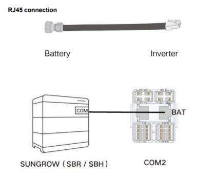
Assemble both the terminator connector and the communication cable to the supplied RJ45 assemblies. Lining up the arrows on the body to the chassis connector, gently push the connectors in until it clicks into place.
