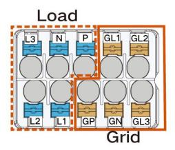
Ensure to connect the cable to the correct input/output. Ensure correct phasing.
