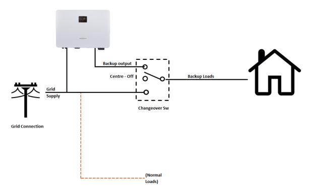
The diagram above is single-phase for clarity, but 3-Phase is exactly the same. If the inverter fails, the owner simply switches from inverter over to grid.
