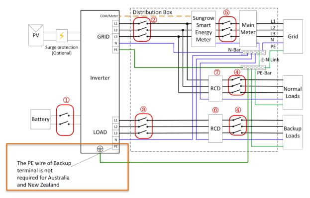
Ensure to connect an earth cable from the chassis to the earth bar, as the earth on the backup connector is not connected.
