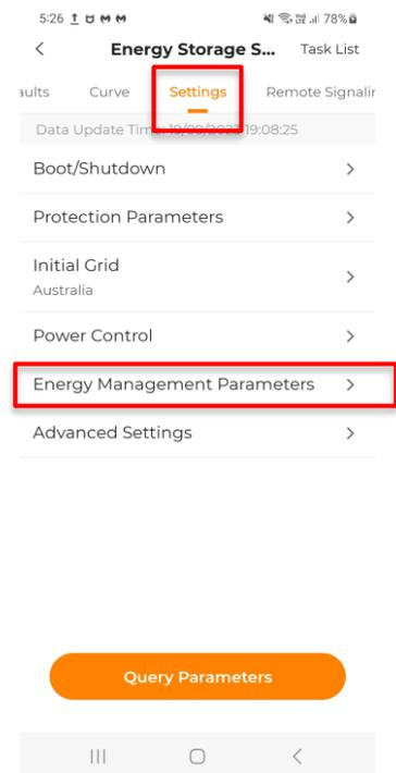
Select “*Forced Charging*”, then enter the start and stop times, and the target charge SOC%.
