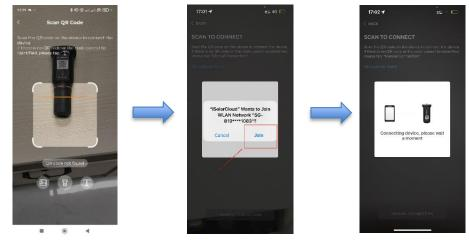
Note: if it requires a manual connection. Click "Go to Set" then connect to the SG network and If it requires a password take note that the password is the Serial number of the WiFi v31 itself. Customer can find the SN on the side of the dongle.
