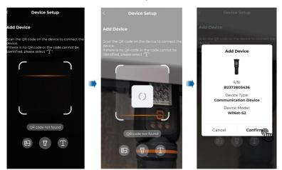
Step 2 Connect the communication device to the home network, so that data can be transferred to the iSolarCloud server over the home network.
