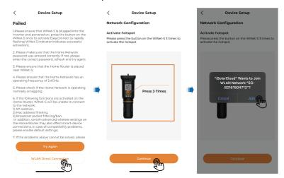
Select the target home network in "Network Configuration" -> enter the password -> wait for the network connection to be established -> complete network configuration.
