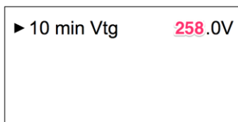
Figure 2 10-minute overvoltage limit
