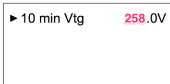
Figure 2 10-minute overvoltage limit
