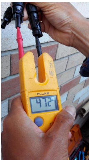
Figure 1 External DC Voltage
