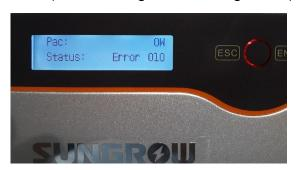
Example fault code = loss of grid voltage i.e. blackout:
