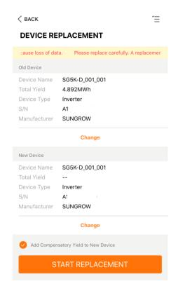
After these procedures are completed, you can conduct replacement and check it on iSolarCloud. The data will be transferred without any abnormal issue.
