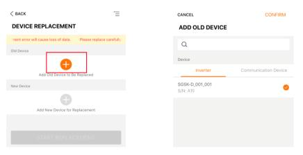
**Step 5**: After you confirm the 'Old Device', the 'New Device' will be availabe to edit. Click Plus icon (+) and you will see the following option. You can scan the QR code on the WiFi device or enter the inverter's serial number manually;
