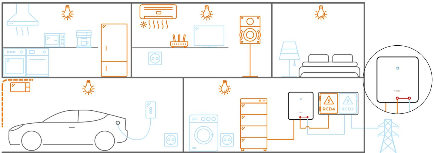
The **bypass switch inside the inverter is closed**. Grid parallel loads (blue) as well as backup loads (orange) are powered by the grid. Both circuits can share the same distribution box but should be protected by their own AC circuit breaker and RCD.
