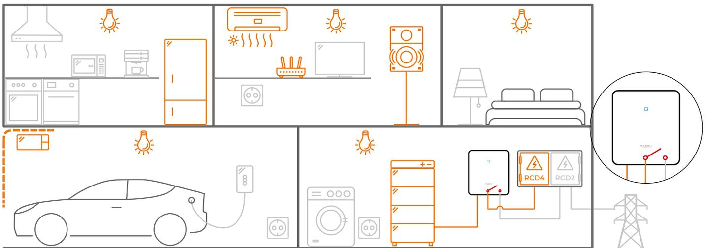
In case of a grid failure the **bypass switch inside the 3-phase Hybrid opens** and **all loads connected to the backup port will get a seamless transition into backup mode**. Only loads not connected to the backup port experience the black out.
