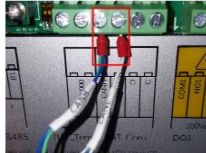
Figure 16: Connection with CANH and CANL into SH5K+ circuit board
