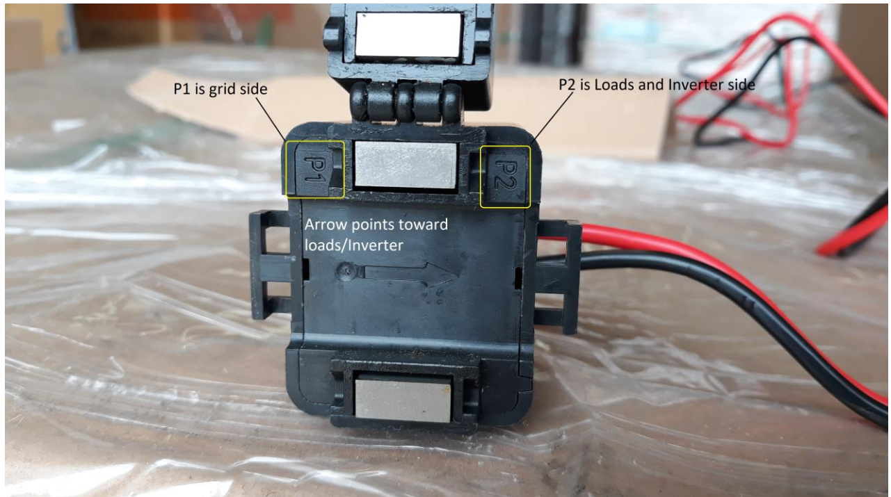
Picture 4 – P1 and P2 polarity with arrow
