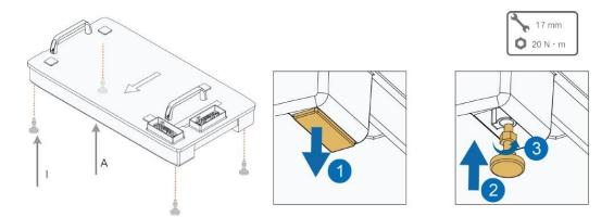
2. Place the base at the acceptable position in right way (arrows outward).
