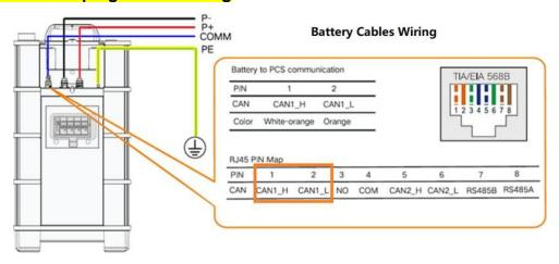
GD\_202111\_Sungrow SBR HV Battery Installation Quick Guide with SHRS \_V2.0
