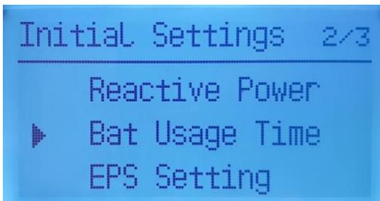
Set battery discharge times (only available if battery connected)
