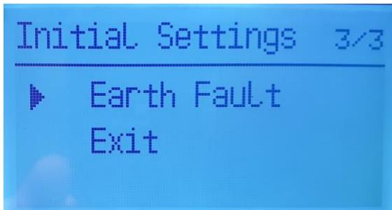
Enter to test Earth Fault alarm
