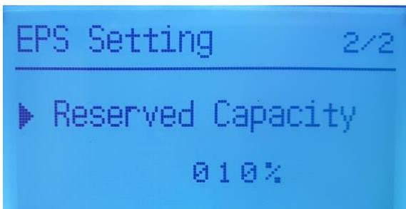
Enter desired value, based on a calculation of total capacity, load, and how long backup is required for.
