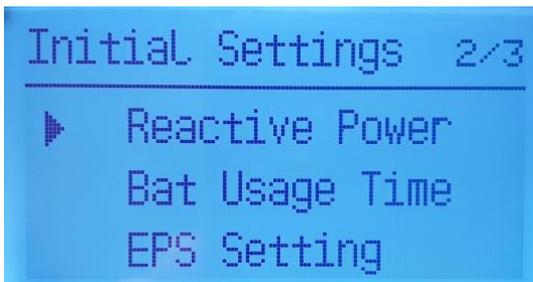
Set Reactive power if required. Note: Grid settings already have State requirements loaded when DNSP selected.
