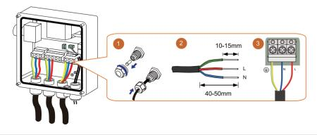
The following figure shows the cable connection between the box and the inverter.
