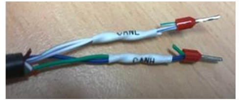
Figure 10 CAN wire with green and green-white pins cutting through
