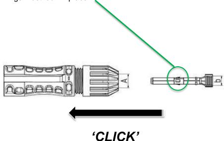
If the pins don't connect properly, the system will show a **703 error**, even if the battery SOC% is shown.
