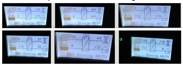
When a customer sees that the energy flows do not add up, the values are normal due to our EMS calculation: Loads = PV +/- battery (discharge or charge) +/- grid power (import or export)
