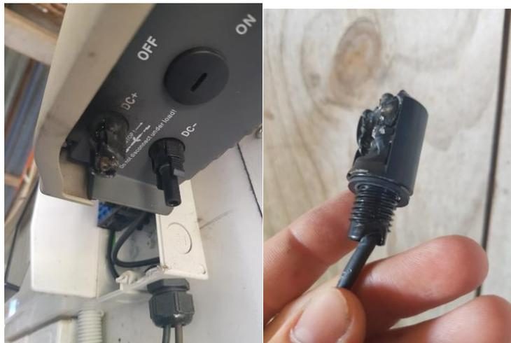
Example of a melted plug
