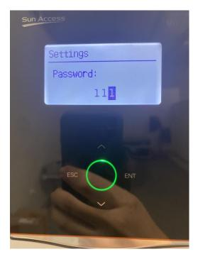
After entering the Setting menu, tap down to the third page which has an **Active Power** function. Enter **Active Power-> Volt-Watt**
