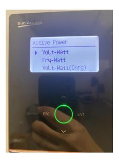
Enable and enter the Volt-Watt function, tap the down button to the second page, you will find the P1-P4 Ref. value. Make sure the percentage is set as the following value (P1: 100% P2:100% P3:100% P4:20%). Then tap ESC button, the inverter will ask if you want to save the setting. Press ENT to save the change.
