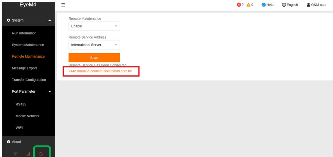
Figure 19 Check the system connecting with iSolarCloud
