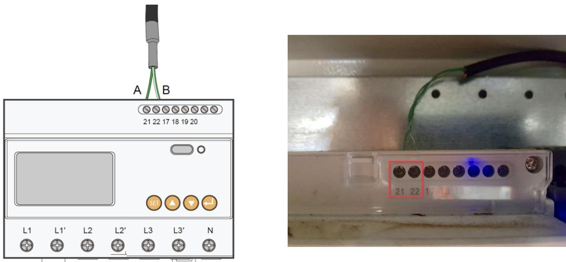
Figure 4 RS485 connections to the energy meter
