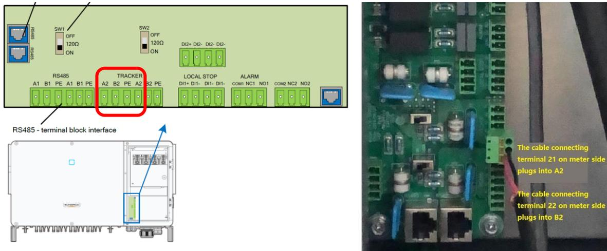
Figure 5 RS485 connections to the inverter
