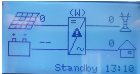
Photo 2 – Dashes showing no battery connected
