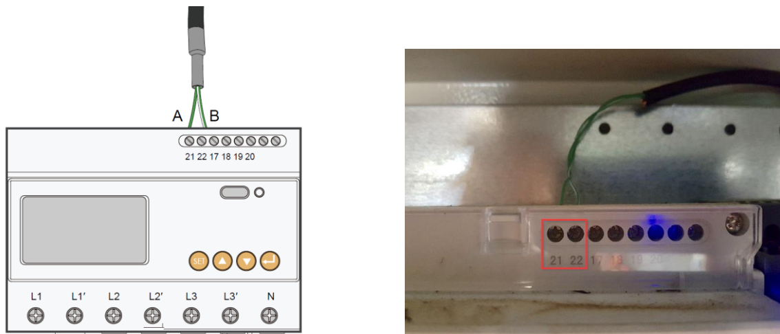
Figure 4 RS485 connections to the energy meter
