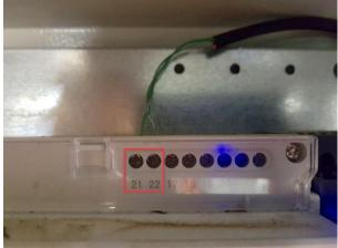
Connect to Logger1000 via the RS485 cable from the energy meter on RS485 port A2 and B2.
