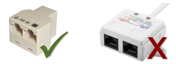
Note: Make sure the splitter splits 8-pin cable into two 8-pin outputs. Some of the splitters only divide 8-pin cables into two groups of 4-pin outputs which will not work.
