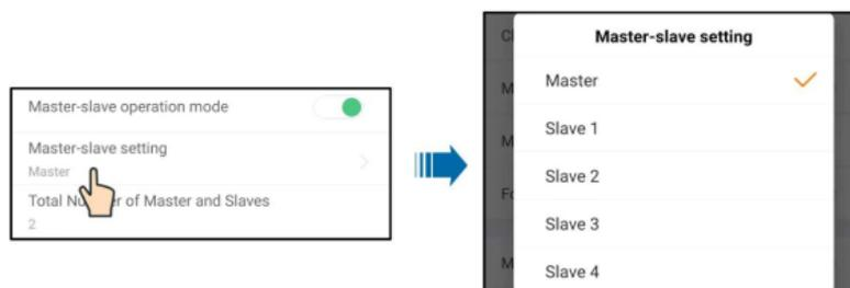
**Step 5** Switch on the "Master-slave operation mode", change the master slave setting to "Master" or "Slave#" correspondingly, and input the total number of master and slaves in the chain.
