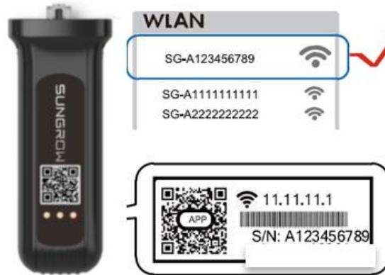
**Step 2:** Open a browser and type 11.11.11.1 into the address bar. Tap “Login” at the top right corner and the password is “pw1111”.
