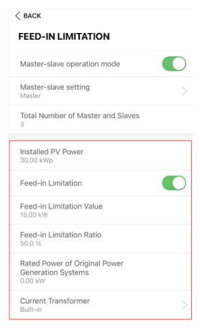
Set total the Installed PV Power to Master inverter – e.g. set 30kW if there are 3 x SH10RT inverters with 30kW PV installed in total.
