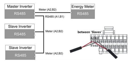
The location of RS485 (A1, B1) and Meter (A2, B2) is shown in the following figure.
