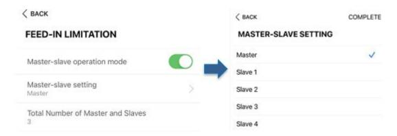
**Step 5** Switch on the "Master-slave operation mode", change the master slave setting to "Master" or "Slave#" correspondingly, and input the total number of master and slaves in the chain.
