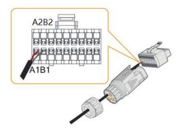
Step 6 Pull the wires outward to check whether they are firmly installed.
